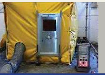
Pressurized Habitat System is an advance safe habitat for hot work localization in a potential area. Pressurized Habitat contains pressurized air that pumps inside the habitat to push other unintended gas outside of the habitat. The system is also attached by inside and outside alarm system and gas detector to ensure safety performance in habitat.
